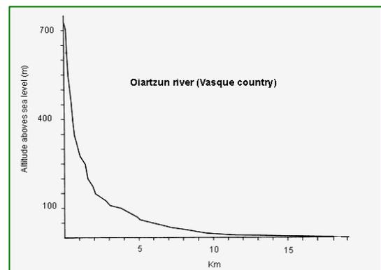
Fig. 1. Longitudinal section of a typical short mountain river.
